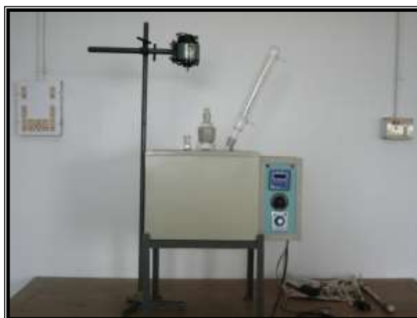
Plate 3.1: 7 litre capacity reactor with oil bath
