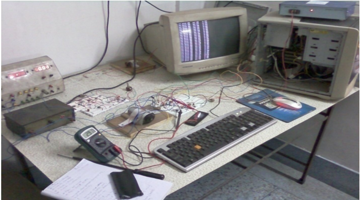
Figure 3.16: Experimental set-up for the speed control of DC motor.
