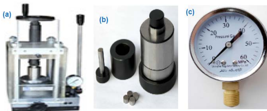
Fig. 5.1. Pellet making instrument (a) Pellet press (b) Dies and (c) Pressure gauge
