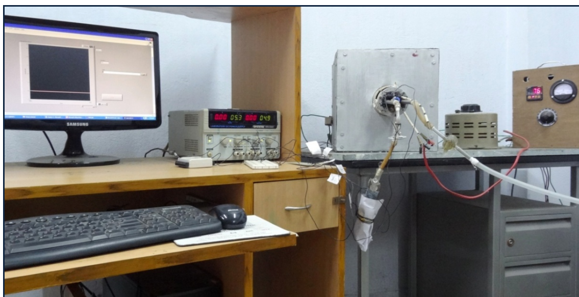
Fig. 5.3. Sensor assembly inside the quartz tube along with allied fittings viz. thermocouple, silica gel tube, inlets for vapours and connecting leads: (a) Customized sensing measurement set-up
