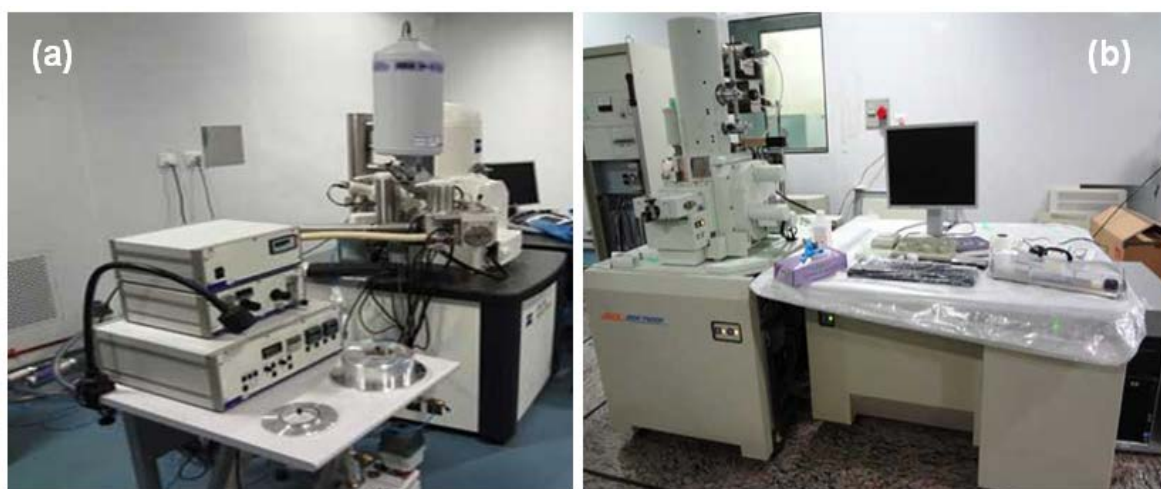
Fig.3.11. (a) SEM instrument with INCA Energy 250 Microanalysis System (EDS), ZEISS EVO-MA 10, (b) FESEM instrument (JEOL, JSM-7600F) PC controlled microscope with INCA Energy 250 EDS at CRNN, CU
