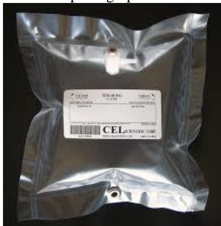
Figure. 4.15. Photograph of Tedlar bag provided by CEL SCIENTIFIC CORP.
