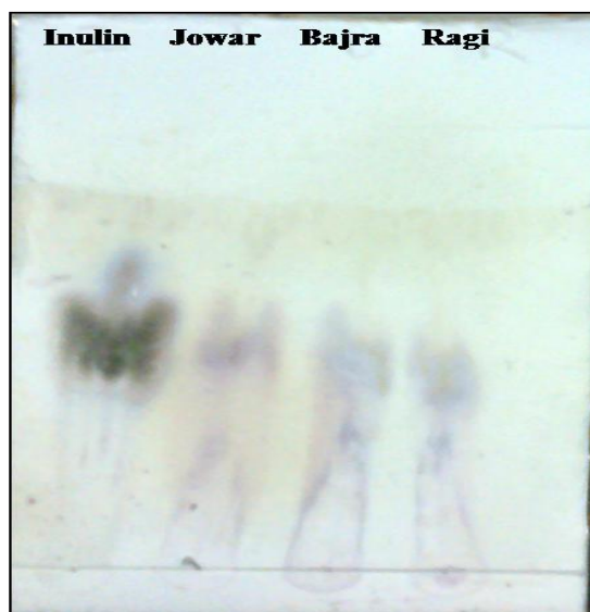
Figure 6.A.2: Silica gel G plate for TLC analysis for (0.2 g or 40%) of hydrolyzed products of prebiotics by oxalic acid
