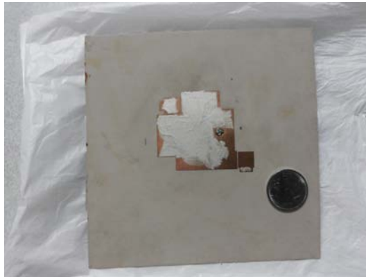
Fig. 7.19 Fabricated prototype of the optimized dual frequency circularly polarized microstrip antenna for vehicular applications
