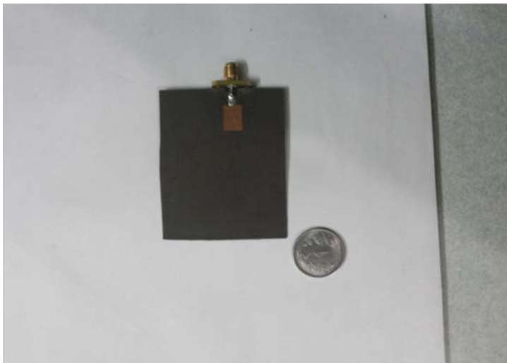
Fig. 7.34(b). Fabricated prototype of the dual frequency circularly polarized grounded slot antenna for WLAN
