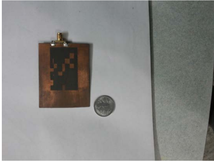
Fig. 7.34(a) Fabricated prototype of the dual frequency circularly polarized grounded slot antenna for WLAN
