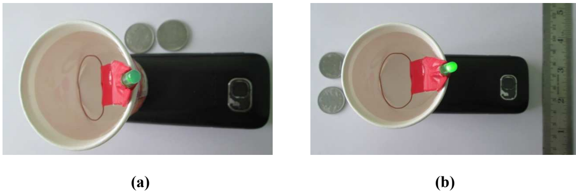
Figure 5.12. Experimental setup for visualizing induced EM field inside water due to non-ionizing radiation from GSM 900 mobile phone (a) not in operating mode and (b) in operating mode.
