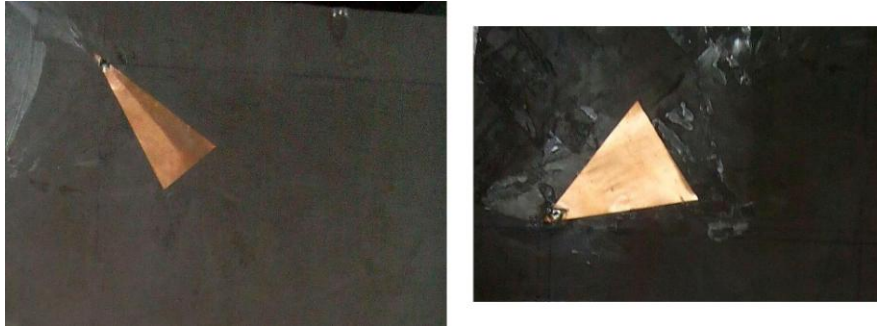
Fig. 6.6 Photograph of fabricated isosceles TMAs: left \theta_i = 77^\circ and right \theta_i = 68^\circ
