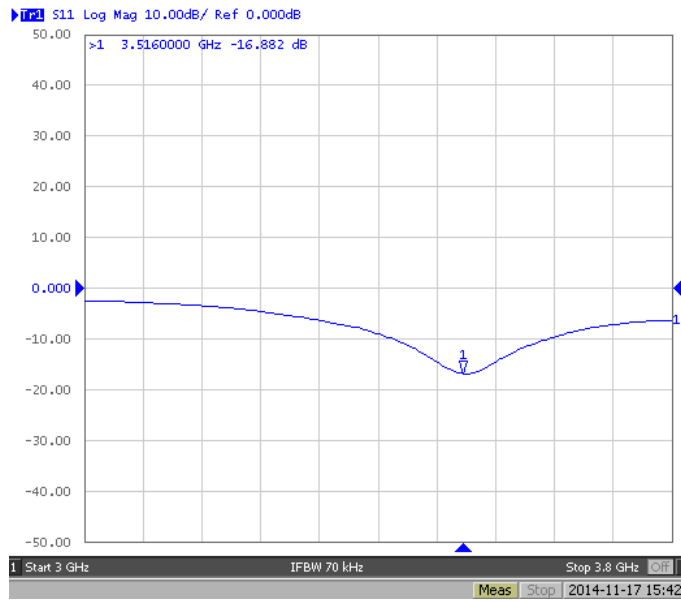
Fig. 12.5 Measured |S_{11}| of sample I of Table II ( a = 25mm, d = 5mm, b_1 = 25mm, b_2 = 17mm, \epsilon_{r1} = 10, \epsilon_{r2} = 25 )
