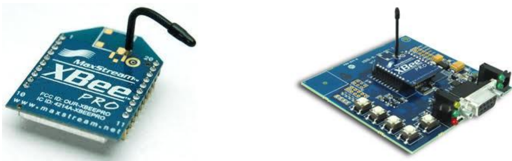
Fig 3.15 Zig-Bee module and board embedded with Zig-Bee module
