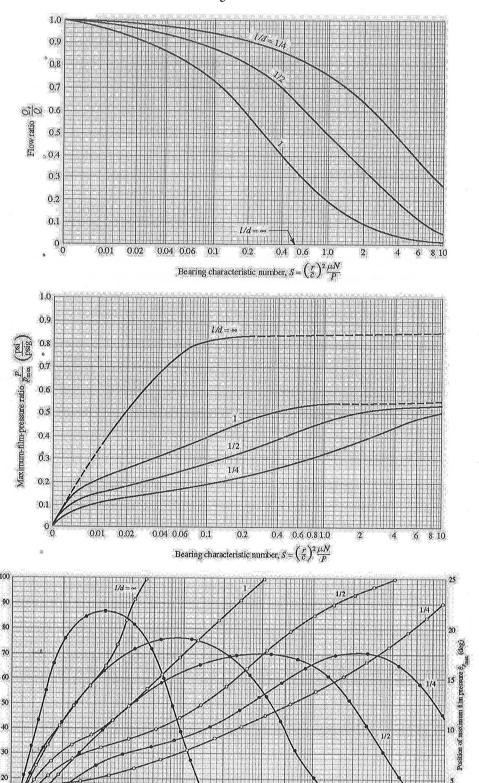
D.08.0.1 0.2 0.4 0.6 0.8 1.0 Bearing characteristic number,  $S = \left(\frac{r}{c}\right)^2 \frac{\mu N}{P}$
