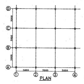
Floor to floor height = 3.5m, Plinth height = 0.6m, Column size = 400mm x400mm
