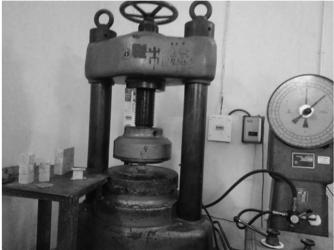
Fig. 4.2 Compressive strength testing of cube samples under progress
