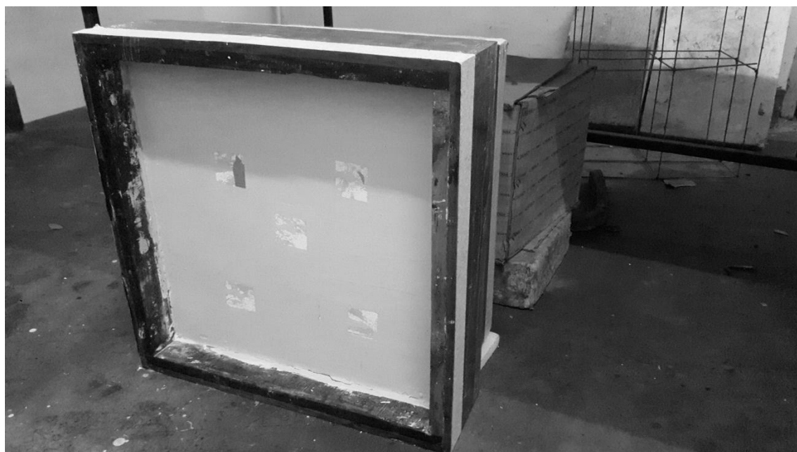
Fig. 3.12 Plastered-puttied-coloured Wall Sample after U-value testing
