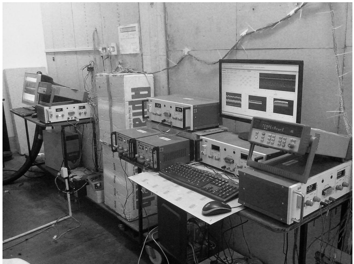
Fig.4.36. Guarded Hot Box test setup with data logging and recording.
