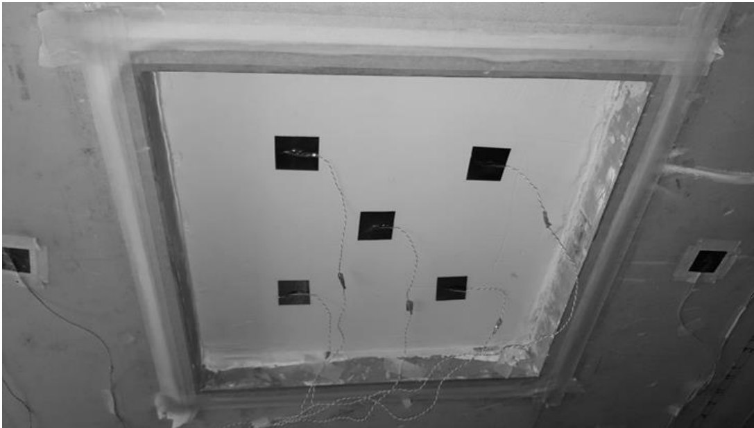
Fig.4.37. Wall sample placed in position with Sensors
