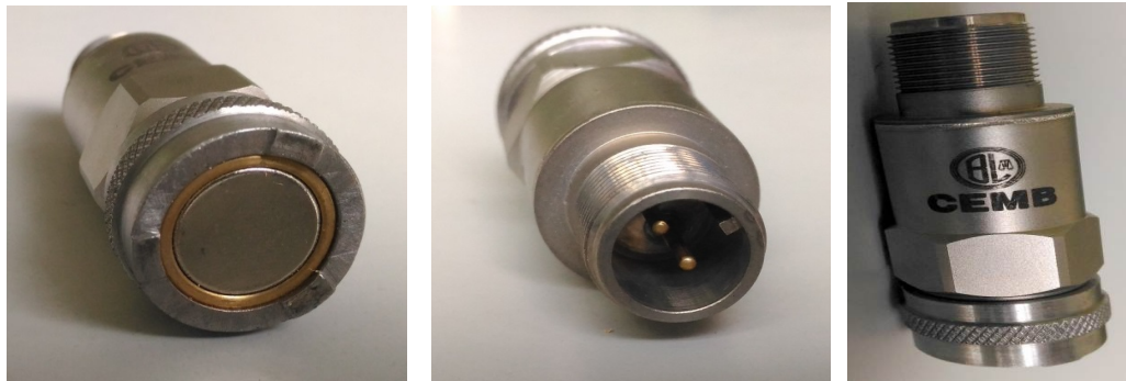
Fig. 4.2.2: Accelerometer in different view.
