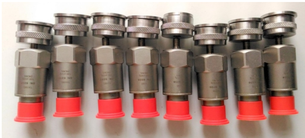
Fig. 4.2.3: All eight accelerometers.
