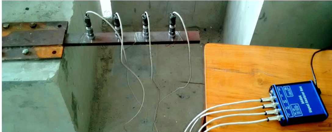
Fig4.2.13: Operational modal testing of undamaged (UD) cantilever beam
