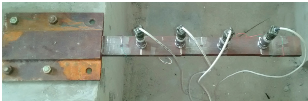
Fig. 4.2.21: During experiment for the steel cantilever beam (double element damage)
