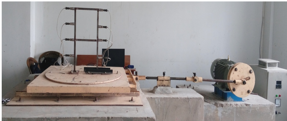
Fig 4.2.28: Full setup for the experiment (Uni directional shake table system along with control panel and motor and experimental portal frame and accelerometers with other accessories)
