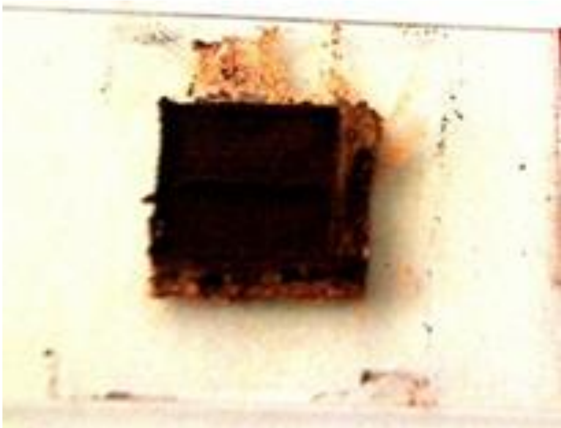
Fig. 3.4: Miniaturized laser sintered part of Copper Powder blended with Silicon Oil
