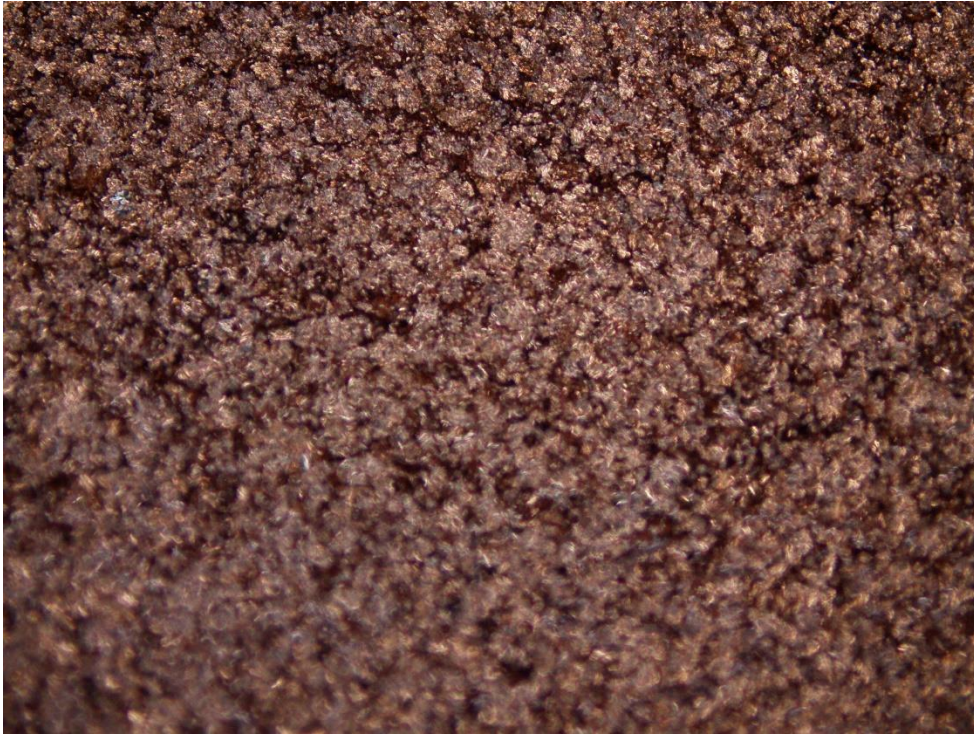
(a) Copper powder with Silicon oil (before sintering);
