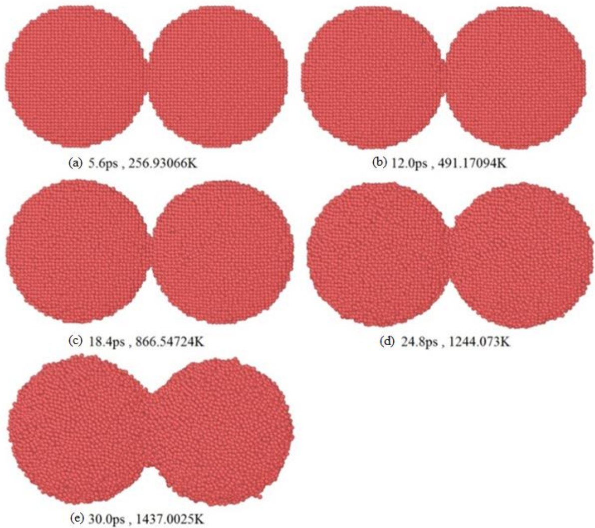
Fig. 2.13: Snap shots of sintering the 2nm nanoparticle pair at time steps 5.6ps, 12ps, 18.4ps, 24.8ps and 30ps
