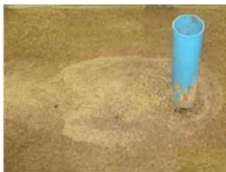
Fig 2.2 Flow situations leading to scour around a vertically mounted cylinder
