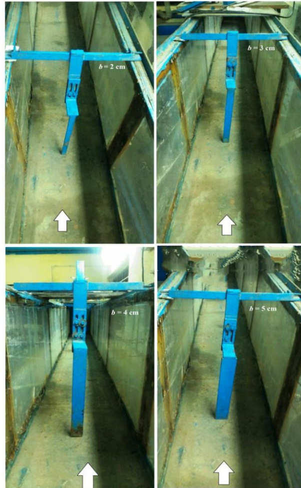
Fig. 3.2 Experimental arrangements of plates b = 2 cm, 3 cm, 4 cm and 5 cm
