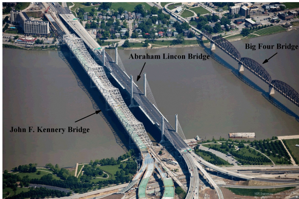
Fig. 1.4 Pier groups of John F.K. Bridge, Abraham Lincon Bridge and Big Four Bridge.
