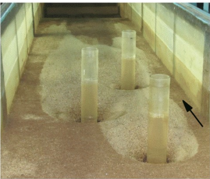
Fig. 3.5. Scoured zones around three identical circular inline-eccentric-inline arranged piers for test nos. 4, 5 and 6.
