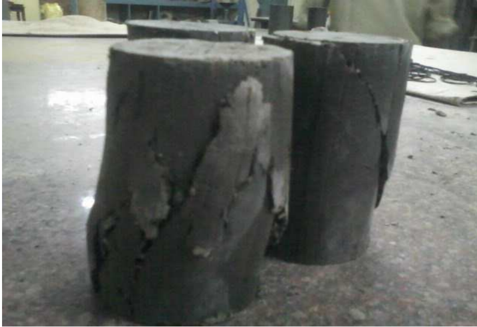
Fig. 3.3: Samples after failure at different confining pressures
