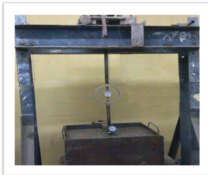
Fig. 4.1B: Set-up for 10 cm model footing tests
