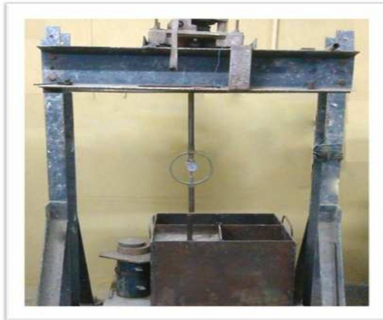
Fig. 4.1A: Set-up for 5 cm model footing tests
