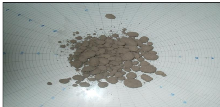
Figure 4.54(h) Specimen GPC-M (failed to form normal specimen)
