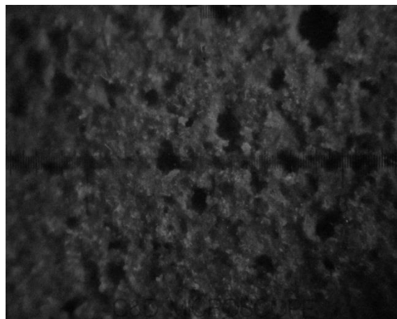
Figure 4.69(a) Specimen GSCB2 showing fresh surface after 1 month exposure to Magnesium sulfate solution
