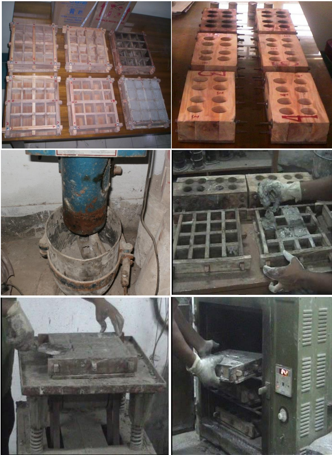
Figure 3.9 Preparation of test specimens
