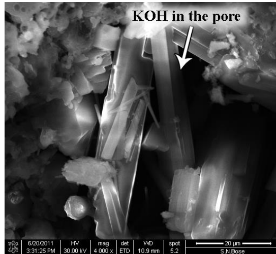
Figure 4.70 (a) SEM @ 4000x zoom of specimen GPC shows crystal structure
