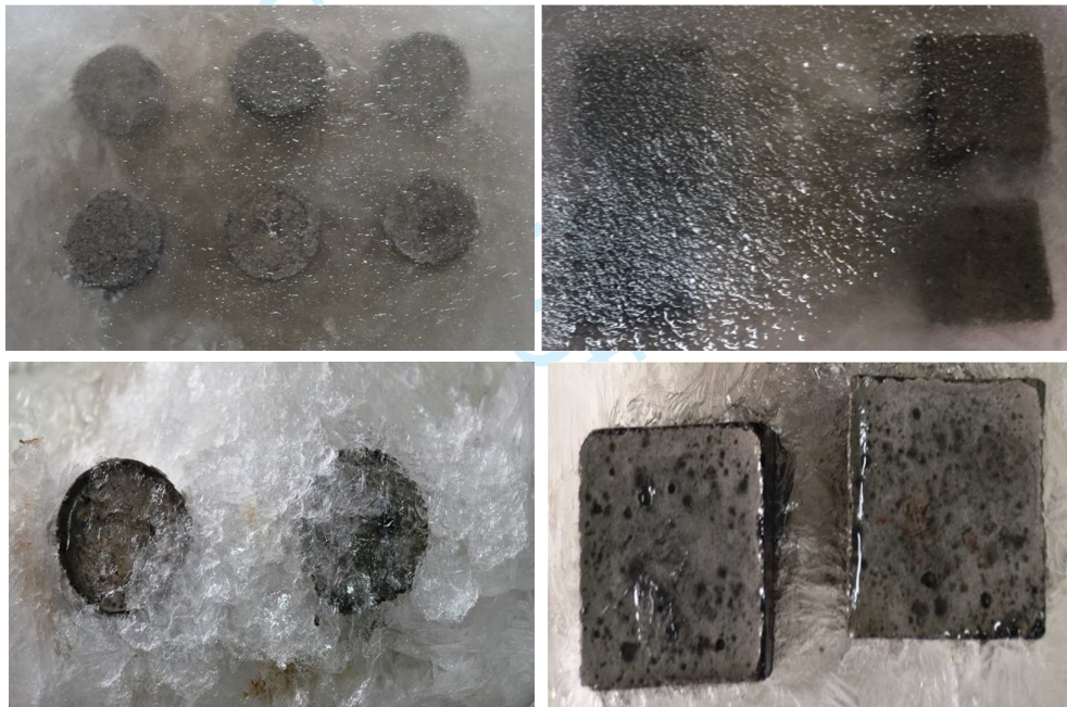
44 Figure 8c. Exposure of specimens to cyclic freezing and thawing 45 46 47 48 49 50 51 52 53 54 55 56 57 58 59 60
