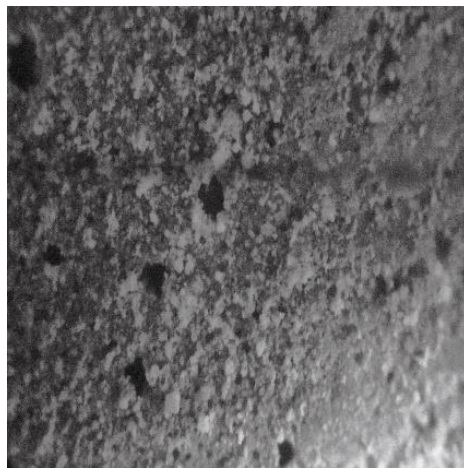
Figure 4.49 (c) Geopolymer paste specimens GL2, after 6 weeks in 10% Magnesium sulfate solution
