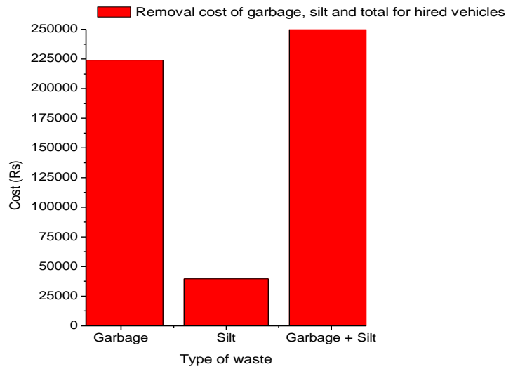
Fig.6.13 Transportation costs of hired vehicles carrying garbage and silt or rubbish
