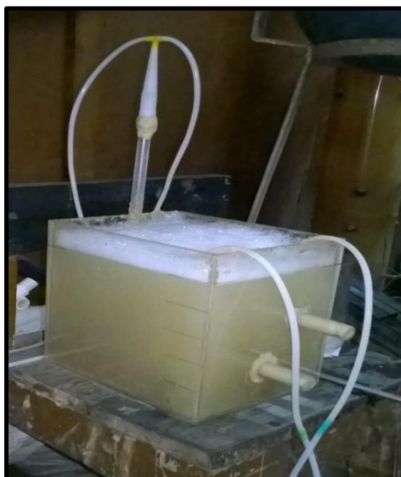
Fig.-8.2: Laboratory scale batch reactor set-up to study performance evaluation of primary treated tannery effluent with isolated pure culture
