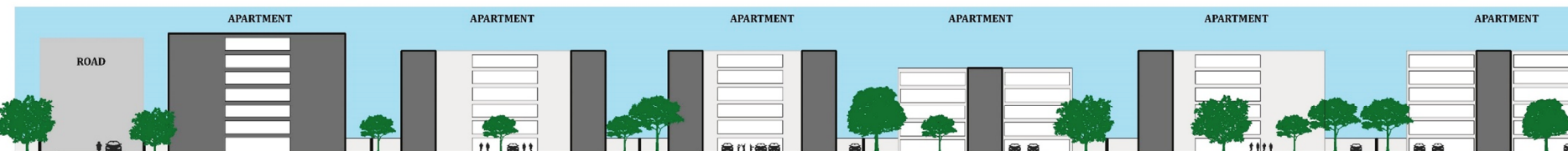
Sector 20 (Panchkula) Central Study Unit opposite Main Neighbourhood Shopping (Primary Roads - 30'-50' or 10-15 m, Secondary Roads - 20' or 6 m) H:W = 1:1, 1.2:1, 1.4:1
