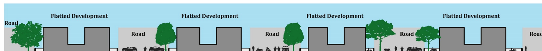
Sector-38 West Study Units with low rise high residential density devoid of Parks (30'- 50' or 10-15 m wide roads) H:W = 1:1.2
