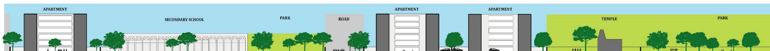
Sector 20 (Panchkula) Inner Study Unit near Park, School and Temple (Primary Roads - 30'-50' or 10-15 m, Secondary Roads - 20' or 6 m) H:W = 1:1, 1.2:1, 1.4:1
