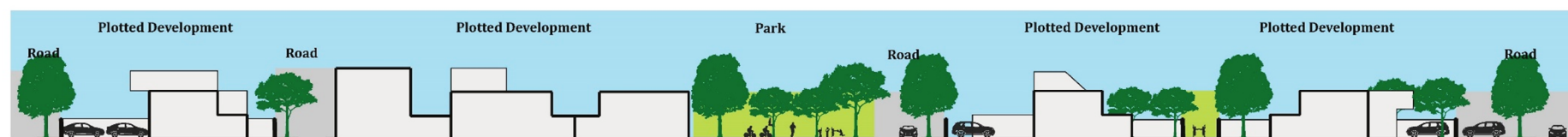
Sector-8 Inner Study Units with low rise low residential density (Primary Roads = 60'- 80' or 18-25 m, Secondary Roads = 40'- 45' or 13 m, Tertiary Roads = 30'- 35' or 10 m) H:W = 1:1, 1:3
