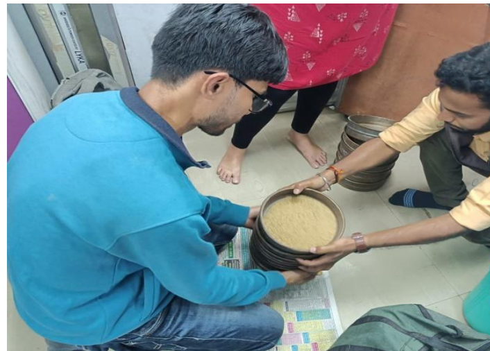
Photograph 1 Analysis of grain-size distribution in the Laboratory of the School of Water Resources Engineering, Jadavpur University
