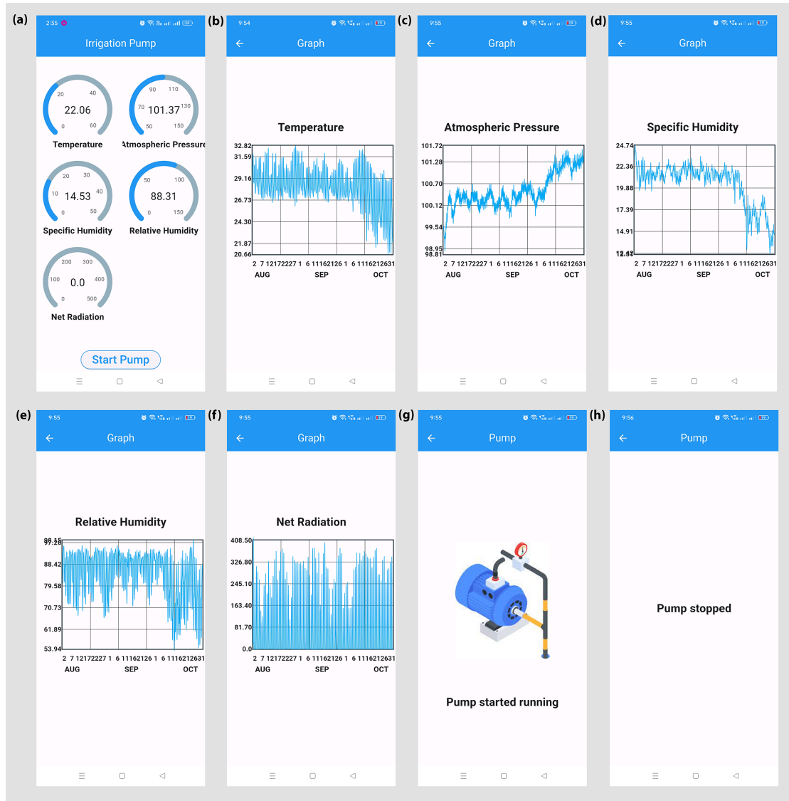
FIGURE 3.9: (a) Home Screen, (b) Graph for Temperature, (c) Graph for Atmospheric Pressure, (d) Graph for Specific Humidity, (e) Graph for Relative Humidity, (f) Graph for Net Radiation, (g) Screen for Pump on, (h) Screen for Pump Off
