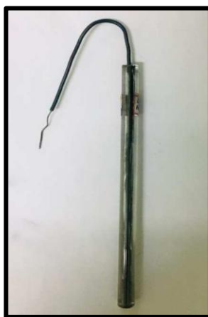
Fig. 2.4: \text{Nd}_2\text{O}_3@\text{GP} working electrode
