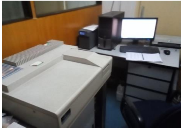
Figure 4.3. Perkin-Elmer Lambda-35 Spectrophotometer.
