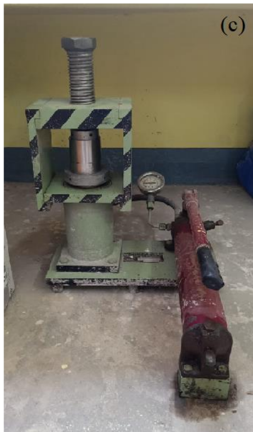
Fig-2.1: Instruments used for sample preparation: (a) Electric Balance (b) Furnace (c) Pelletizer
