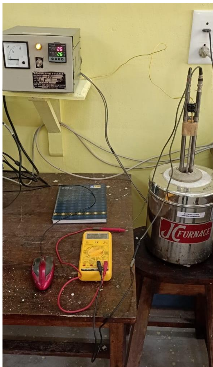
Fig-2.4: DC conductivity measurement experimental setup
