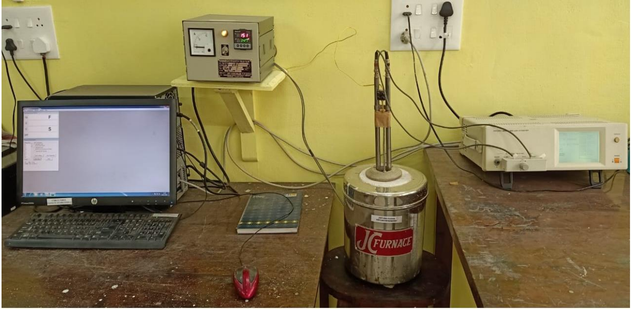
Fig-2.5: AC conductivity measurement experimental setup
