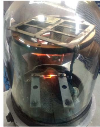
Fig. 6.5(c) \text{ZnTe} by thermal deposition
