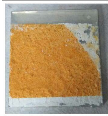
Fig.6.5(b) Deposited \text{SnI}_2 by Thermal Evaporation
