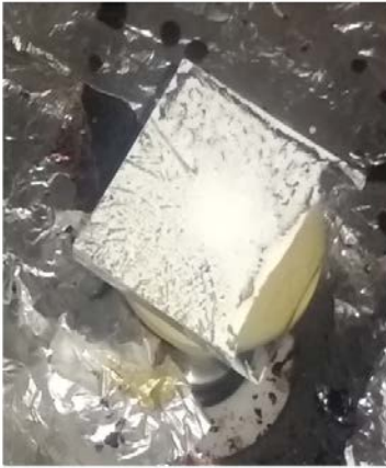
Fig. 6.5(a) Spin coating of \text{TiO}_2
