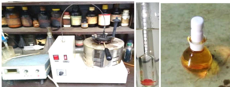
Figure A1.1: Flashpoint tester, hydrometer and Specific gravity bottle
