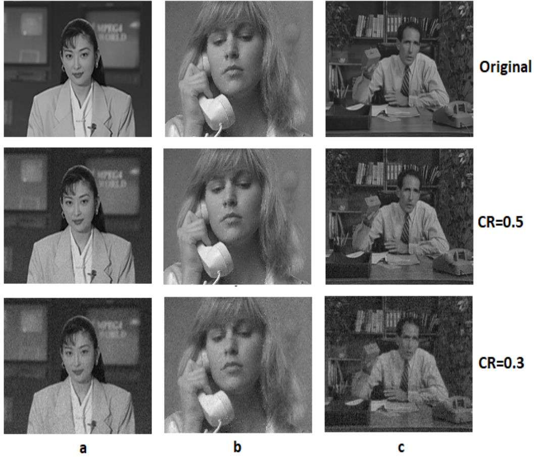
Figure 4.13: Quality of different recovered video frames for two CR values for three different video - (a) Akiyo (b) Suzie and (c) Saleman
