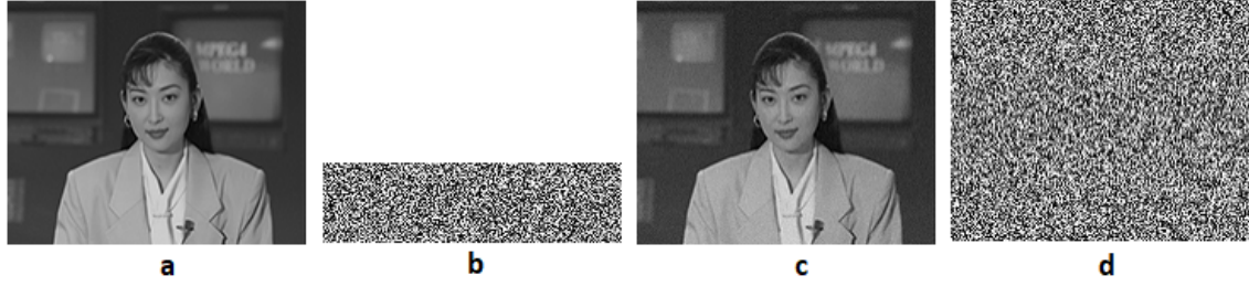
Figure 4.10: Key sensitivity test with Akiyo video (a) Original frame (b) Compressed and encrypted frame (c) recovered frame using exact key (d) recovered frame using a key that differs by one bit from the exact key
