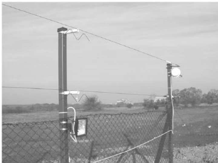
Fig. 2.8: Sinusoidally curved wire antennas deployed in security fence radar [86]. ©IEEE
