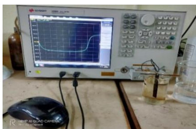
Fig. 2.8. Experimental Testing setup: impedance analyzer connected with the electrode.
