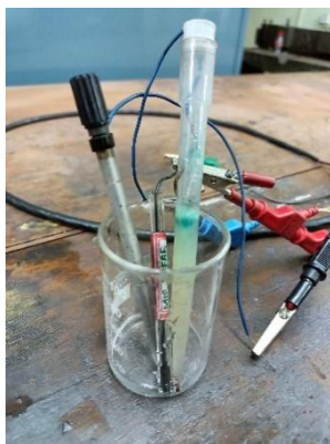
Fig. 6.4. A traditional three-electrode system setup, illustrating the separate, manual positioning of the working, Ag/AgCl reference, and platinum counter electrodes, which introduces variable uncompensated resistance due to positional errors.
