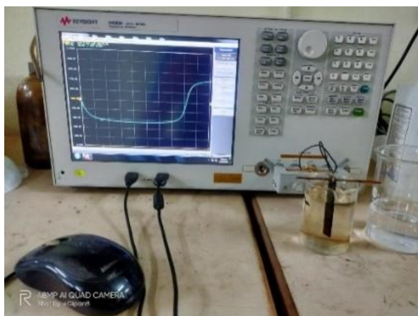
Fig. 5.3.2. Experimental Testing system – electrode coupled with the impedance analyzer.
