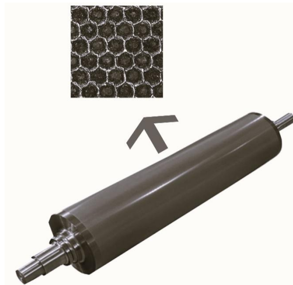
Figure 1.2: Schematic diagram of anilox roller [25]
