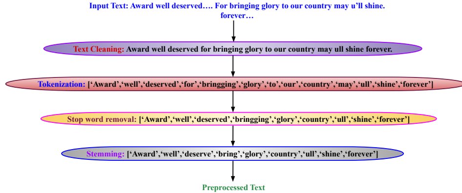
FIGURE 2.2: Steps with result of the text preprocessing of PSA text System.
