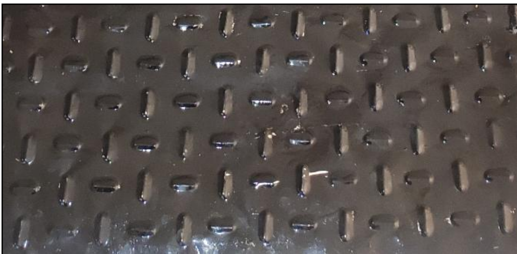
Figure 5.1 : Actual absorber plate having semi-capsule protrusions
