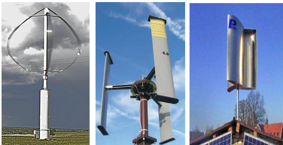
Figure 1.12 (a) Darrieus vertical axis wind turbine (VAWT) (b) H-rotor Darrieus VAWT (c) Savonius VAWT (Mahmoud and Xia, 2012)
