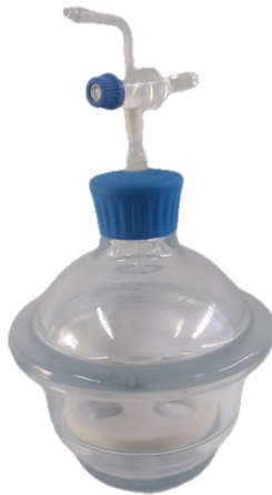
Figure 11 Glass desiccator for sulfur dioxide gas exposure
