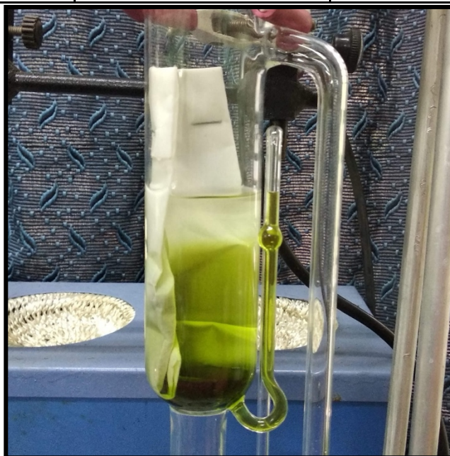
Figure 9 Thimble of Soxhlet extractor showing extracted compounds from leaves
