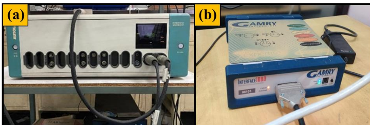
Figure 3.3: (a) Autolab PGSTAT (M204) and (b) Gamry Interface 1000 instrument diagram.
