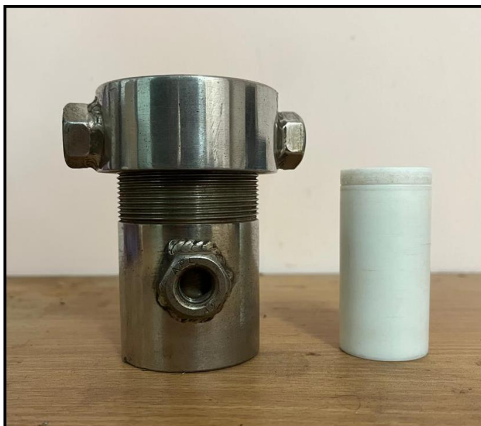
Figure 3.2: Image of a teflon lined autoclave.
