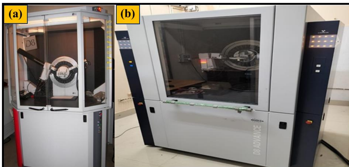
Figure 3.4: Image of X-rays diffractometers (a) D8 Advance Bruker set-up and (b) Rigaku MiniFlex 600 set-up.
