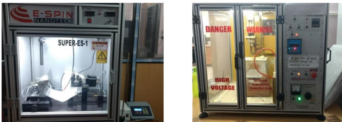
Figure 4. 6 Electrospinning Machine used for nanofiber fabrication (E-spin Nanotech, Kanpur, India)
