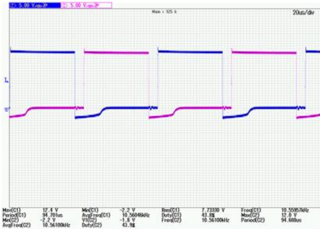
Figure 2.19: H-bridge driver output voltage at 10 kHz with 43% duty cycle.
