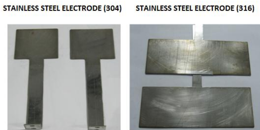
Figure 3.33: Stainless steel electrodes (SS 304, 316).
