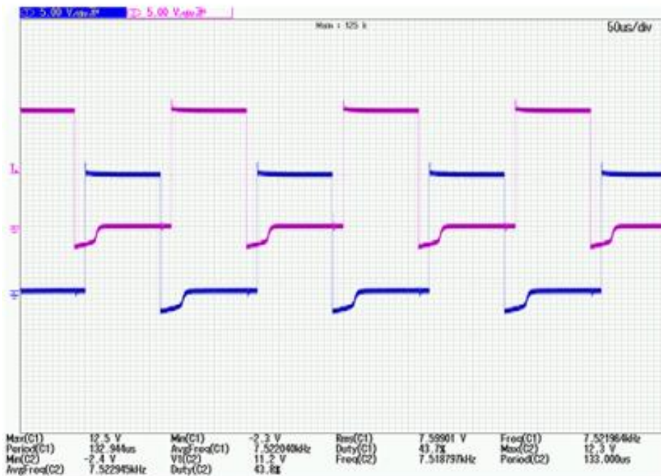
Figure 2.18: H-bridge driver output voltage at 7.5 kHz with 43% duty cycle.
