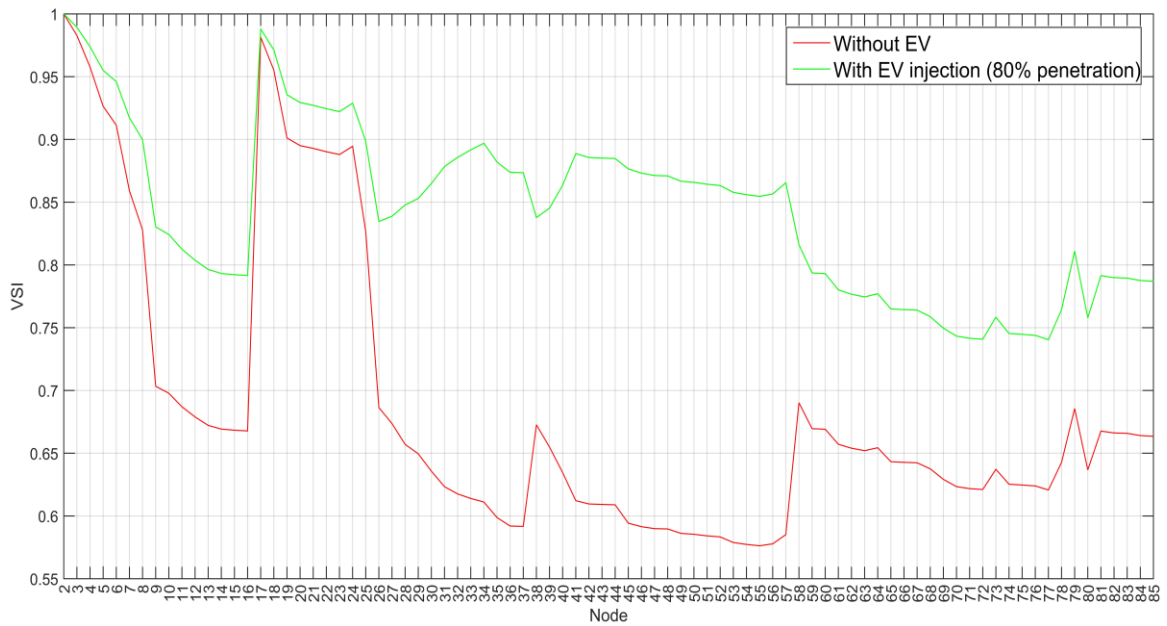
Fig. 4.1.14. VSI improvement characteristics (Case: Without EV & 80% EV penetration at IEEE 85 bus) under the Case-Study# 4.1
