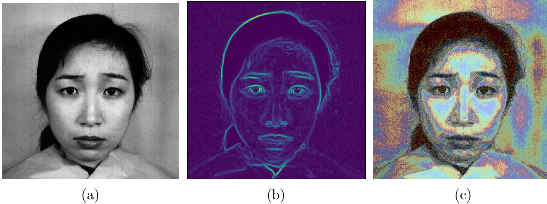
Figure 3.4: "Preprocessing by our Models on a sample image from the Jaffe Dataset ": (a) Original Image, (b) Sobel Edges of Image, (c) Lateral Normalized Image
