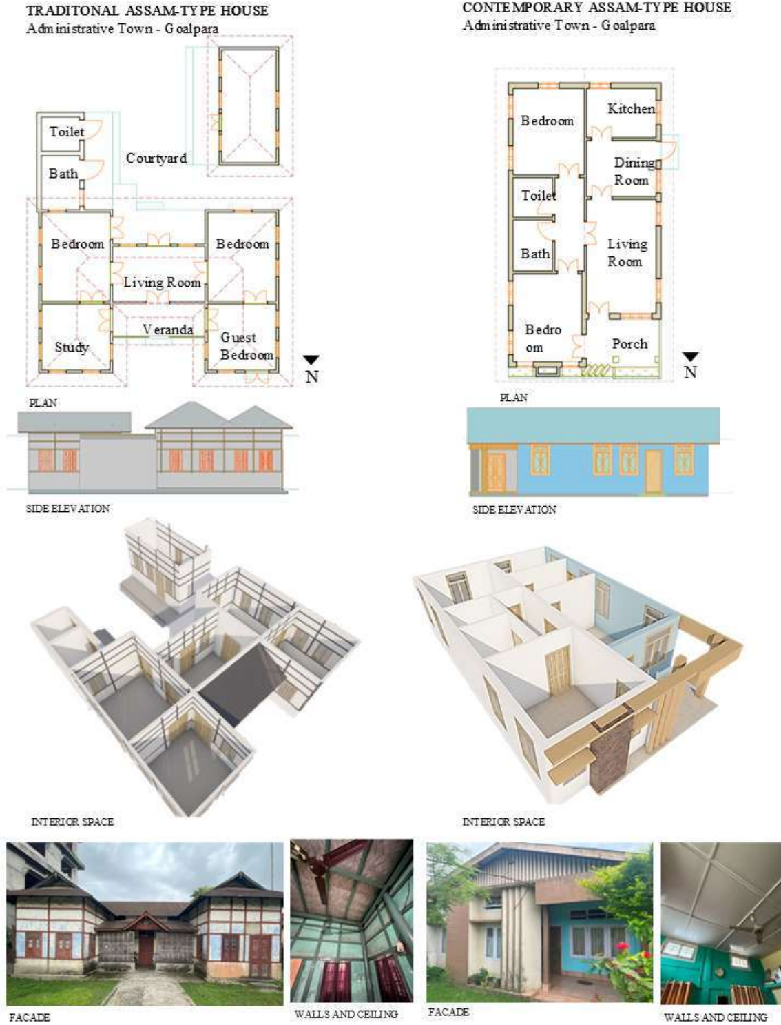
Figure 4.17: Plan, Elevation and Interior View of a Traditional Assam-Type House and a Contemporary Assam-Type House at Goalpara, Assam (Source: Author)
