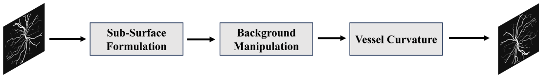
Figure 2.3: Block Diagram of the Vessel Curvature-based Fundus Image Augmentation
