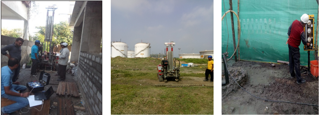
Figure: 2.0 Representative Photograph of DMT, CPT and PMT tests at site-3 (RJ), Site-4 (HA) and Site-9 (VT) respectively
