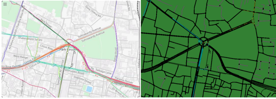
Figure 4.17 Open Street Map of the Simulation Area and Imported Version in SUMO
