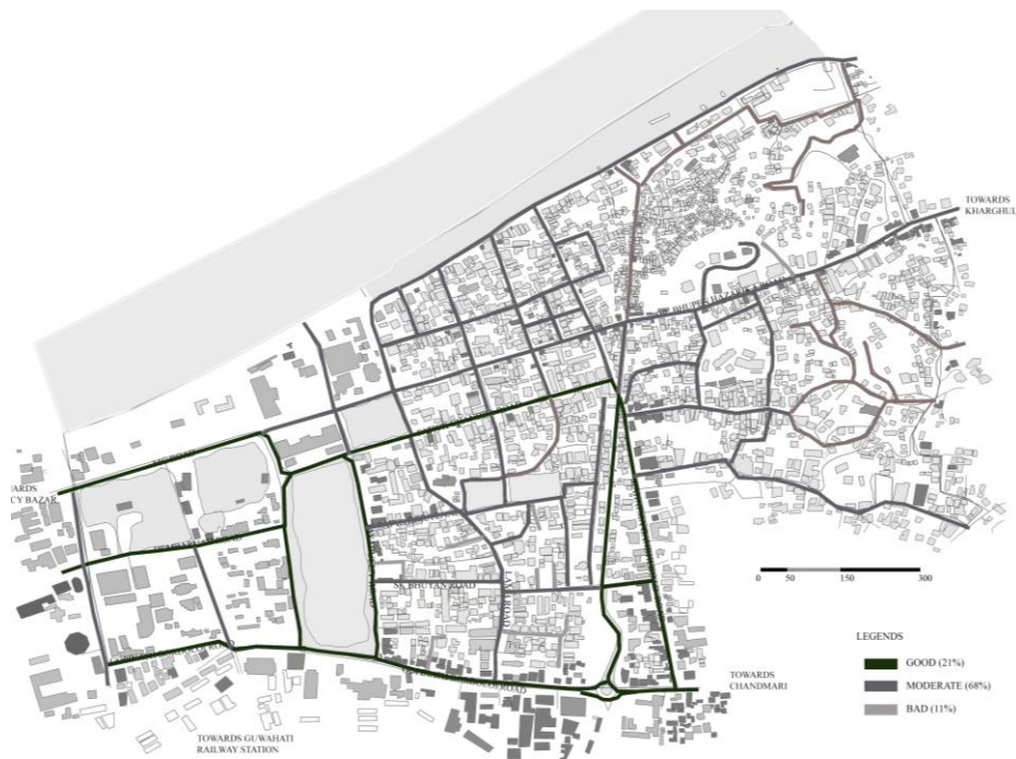
Fig. 5.23: Surface Condition of Roads in Uzan Bazar
