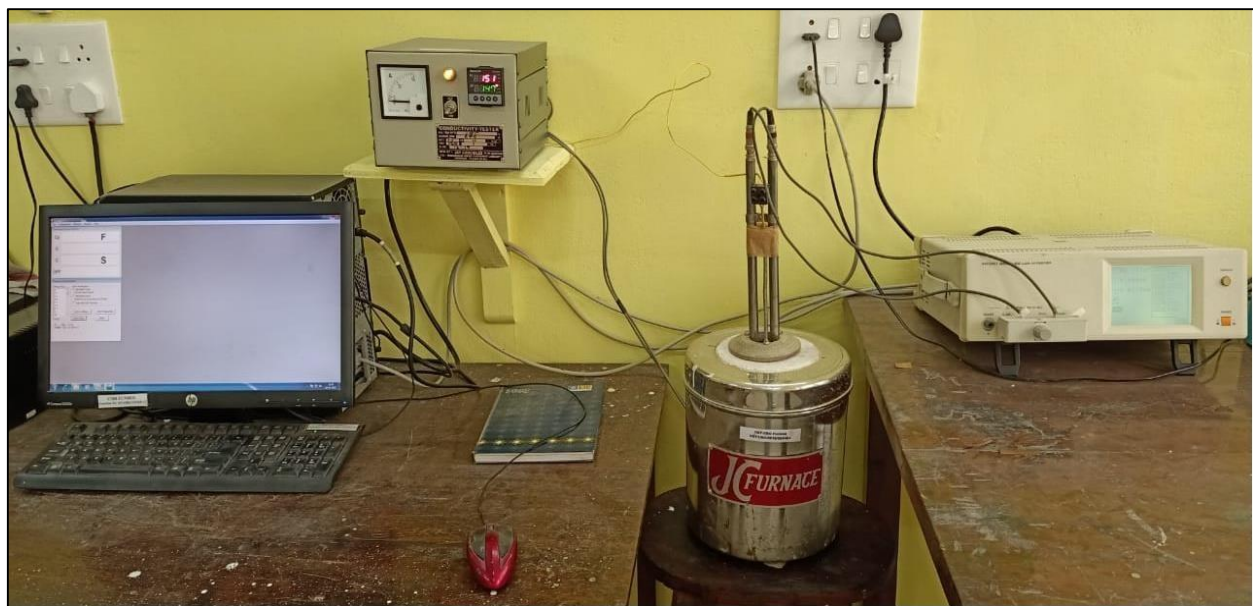
Fig. 2.5 AC conductivity measurement set up
