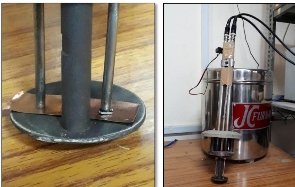
Fig. 2.3 Two-probe method set up
