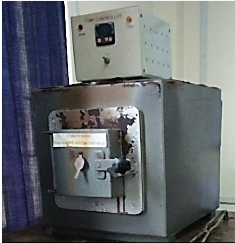
Fig. 2.1 (c) Heating the Mixtures in High Temperature Furnace
