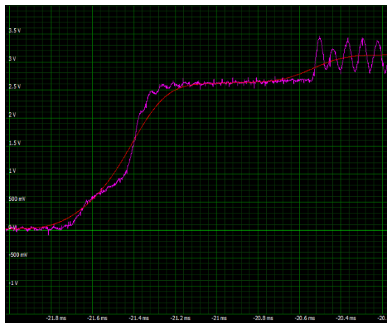
Fig. 4.8 Voltage vs. time signal after noise reduction (red)
