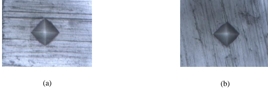
Fig. 2.3 Vicker hardness impression of (a) RHA, and (b) Projectile steel
