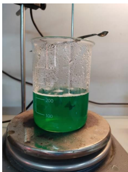
Figure 4.1: Schematic representation of setup for electroless nickel deposition
