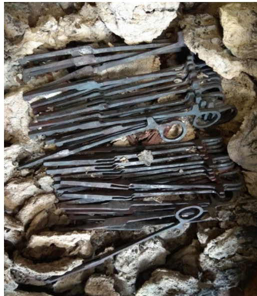
Figure 1.3: Annealing process at Baruipur in cow-pat furnace
