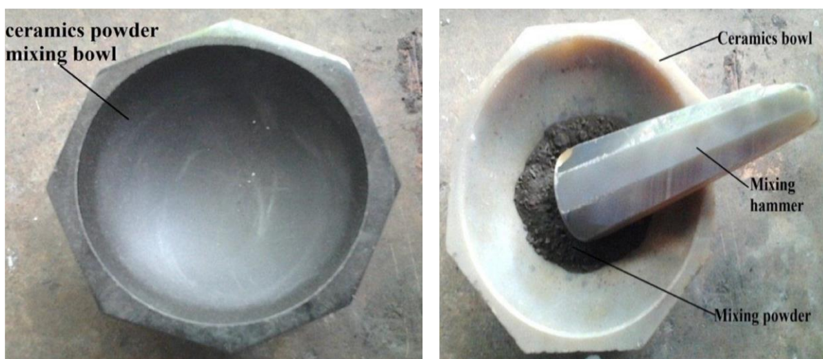
Figure: 3.1b) Ceramic powder mixing bowl and mixing hammer
